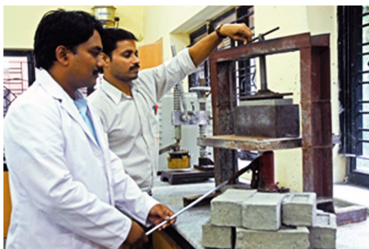
Photos 35 and 36. Laboratory production and sample brick
